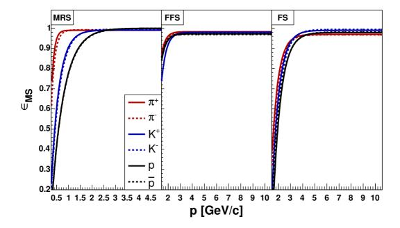
Figure 4.22: Fitted correction functions for multiple scattering. The mid-rapidity panel shows results obtained for 90° with D5 set at a current of 350 A and B polarity. The results for the forward arm are obtained with D1 set at 676 A, and with the FFS positioned at 8° and FS at 4°.
