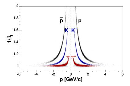
Figure 4.13: The identity of the particles becomes apparent when correlating the  $1/\beta_t$  from TOFW with p determined from bending of the particles' trajectories in the magnetic field of D5.
