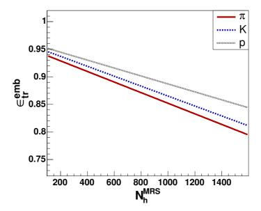
Figure 4.19: Results of tracking efficiency in the MRS as determined by embedding simulated TPC hits into real data. The unit along the abscissae is the number of real TPC hits per event in the spectrometer, i.e. the sum of hits in TPM1 and TPM2.
