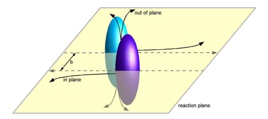
Figure 1.6: Simplified picture of a non-central heavy ion collision indicating the directions of in-plane and out-of-plane flow components. b denotes the impact parameter.
