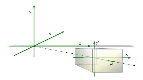
Figure A.1: Illustration of coordinate systems defined for the BRAHMS experiment. The global unprimed coordinate system has z direction along the beam pipe and is centered at the nominal interaction point. The primed system exemplify the local coordinates of a tracking detector in the forward arm.
