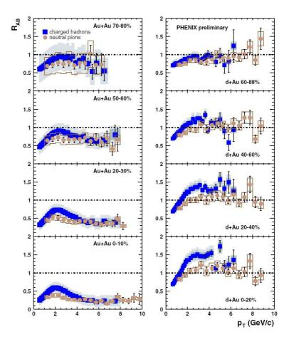
Figure 1.17: The results from PHENIX on the nuclear modification factor for charged hadrons and neutral pions in Au+Au (left panels) and preliminary results for d+Au [86]. High  $p_T$  particles in Au+Au collisions are more suppressed with increasing centrality, while the opposite trend is seen for d+Au.
