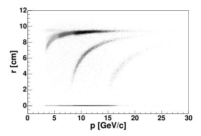
Figure 4.16: Radii of detected Cherenkov light rings plotted against the corresponding momenta for positive particles. The different shades correspond to three different magnetic field strengths with the forward arm located at 4°.
