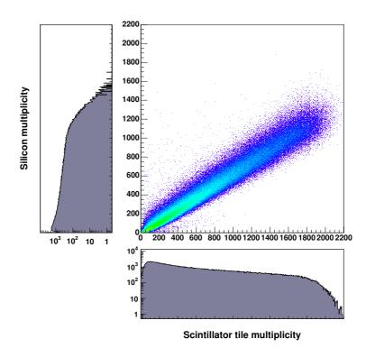
Figure 3.5: The correlation of the multiplicity as determined by the silicon and tiles in the multiplicity array (big panel). The individual distribution of Si (left) has a somewhat lower upper limit than the one for the tiles (bottom). The reason for this difference is attributed to different Landau distributions of energy depositions in the two barrels and a slightly higher probability for saturation in the readout electronics of the scintillators.
