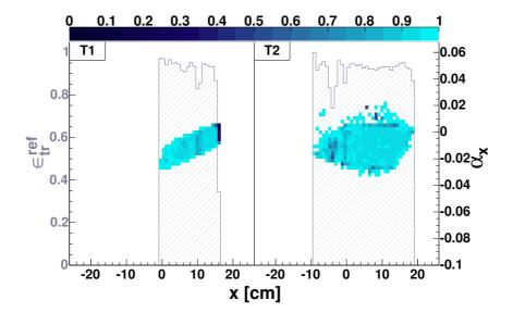
Figure 4.20: Results for tracking efficiency in T1 and T2 obtained with projecting reference tracks. The efficiencies shown are deduced with FS operated at 3° and with magnets at A polarity with magnet current of 1692 A. The axis on the right hand side shows the x component of the detector track slope corresponding to the front histograms, while the left axis is the scale of the rear plot.
