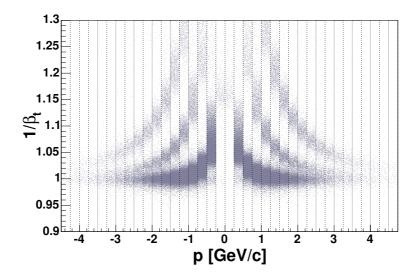
Figure 4.14:  $1/\beta_t$  plotted vs p for particles with  $\eta \in [0.9, 1.1]$  detected by the MRS. The binning along the momentum axis was chosen wide enough to have enough statistics for fitting functions to each momentum bin's distribution in  $1/\beta_t$  and narrow enough so that this distribution is approximately described by a triple Gaussian.
