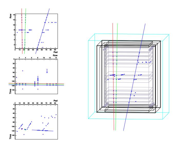
Figure 4.2: Three track segments are reconstructed from hits in T1. The left panels show two-dimensional projections on the axes of the TPC.
