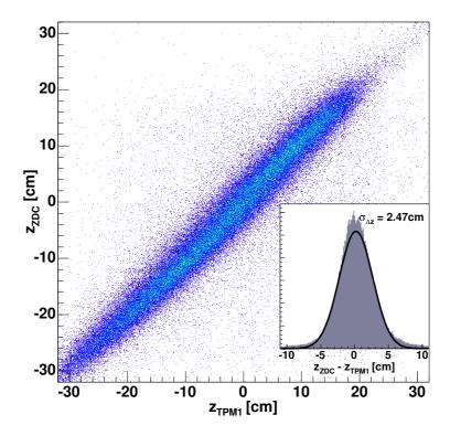
Figure 3.7: Correlation of vertex determined using ZDC and from projecting tracks in TPM1 to the beam axis. Due to worse timing resolution in the ZDCs relative to the BB counters the vertex resolution is not as good as in fig. 3.6.
