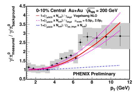
Figure 1.14: Excess of photons in central Au+Au collisions at  $\sqrt{s_{NN}} = 200\,\mathrm{GeV}$  as determined by the PHENIX experiment. The lower dot-dashed curve indicates the expected enhancement if there was no suppression of mesons in the medium.
