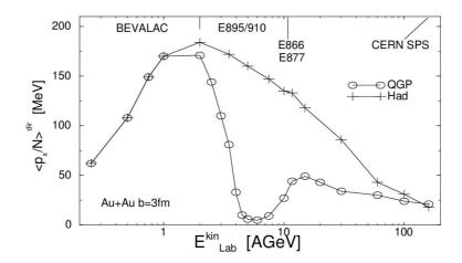
Figure 1.7: Directed transverse flow excitation function in a hydrodynamic picture with and without at QGP phase transition [19].
