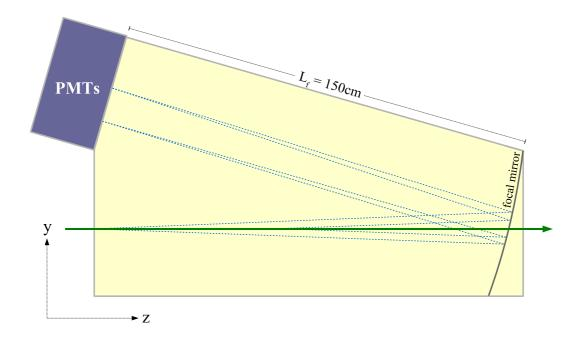
Figure 4.6: Ring generation from a particle traversing the RICH. The dashed lines indicate the direction of photons in the induced shock wave.
