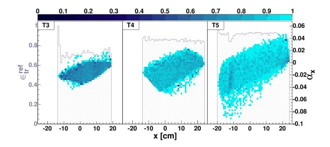
Figure 4.21: Results for tracking efficiency in T3, T4 and T5 obtained with projecting reference tracks. The correspondence of axes to histograms is as in fig. 4.20, as is the spectrometer setting.
