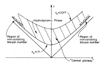
Figure 2.5: The longitudinal evolution of a heavy ion collision according to Bjorken [106]. One-dimensional hydrodynamic expansion start after an initial time  $t_0 \sim 1 \,\text{fm/c}$ . The net-baryon number is found close to the asymptotic t = z line.
