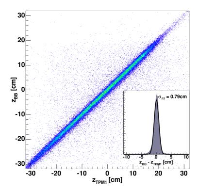
Figure 3.6: Correlation of the location of the primary vertex determined from BB timing difference and from reconstructed particle tracks in TPM1 projected back to the beam line. The main component in the width of the distribution is the timing uncertainty.
