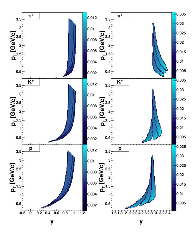
Figure 4.18: Several acceptance maps generated with  $z \in [0,5]$  cm for the MRS at 40° (left panels) and the FS at 4°. The different maps for every particle species correspond to three different magnetic field settings in each spectrometer. All the maps are obtained with the spectrometers at B polarity, which for the FS exclude negative particles. The darker central bands in the MRS maps indicate lower acceptance where particles hit bad slats in TOFW.
