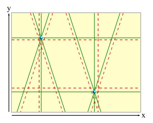
Figure 4.3: Projection image of two particles traversing a DC modules and generating hits in the anode wires. The location of a track's hit in a module corresponds to the intersection of four solid lines. The dashed lines indicate false position components before the left-right ambiguity is solved.
