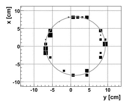
Figure 4.7: The hits generated in the PMTs of the RICH are lying on circular circumference. A ring is fitted to the PMT hits and its radius calculated.
