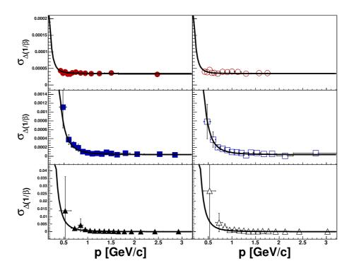
Figure 4.11: Time-of-flight resolution fits for TOFW. Pions (upper panels), kaons (middle) and protons are well fitted with eq. 4.18. The left (right) panels show positively (negatively) charged particles.
