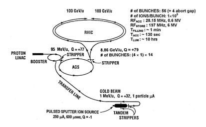
Figure 3.2: Stepwise acceleration in the RHIC complex.
