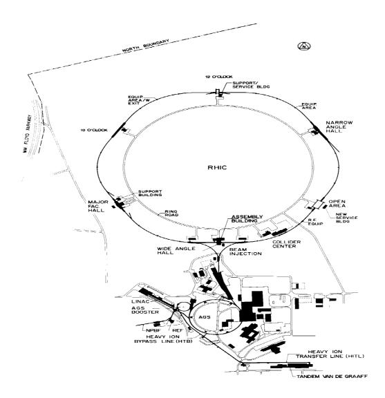
Figure 3.1: Overview of the heavy ion accelerator complex at BNL.
