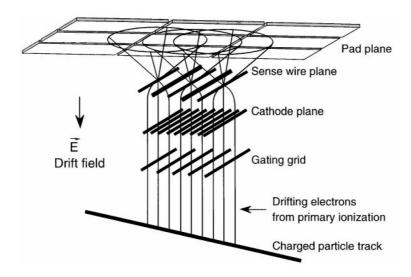
Figure 3.8: The layout of the proportional chamber region of a TPC. The BRAHMS TPCs are located outside magnetic fields and the tracks are therefore straight lines. The drawing was taken from [122].
