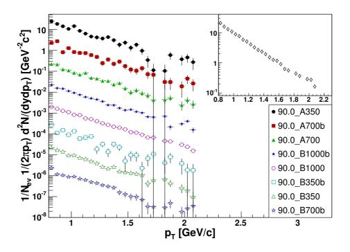
Figure 4.26: Invariant  $p_T$  spectrum values obtained for negative pions around y=0 all scaled by 0.1 relative to the spectrum above. The small panel is the weighted average of the spectra at each setting, for which the weight of each bin is the inverse statistical error. Only  $p_T$  bins where all settings have non-zero values are shown.
