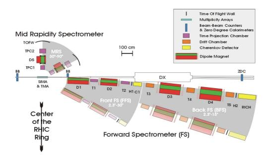
Figure 3.3: Birds-eye view of the BRAHMS experimental setup consisting of two rotatable spectrometer arms and global detectors.
