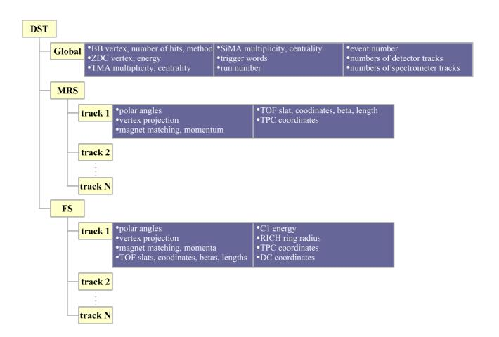
Figure 4.8: After global tracking and ID detector matching the data is organized into DST structure for easy and fast analysis.
