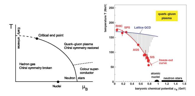
Figure 1.3: The phase diagram of QCD matter. In the left panel the solid line indicates model estimates for the first order phase transition, while the long-dashed line outlines the region for crossover. The short-dashed line shows the phase transition between normal and super-conducting QGP (not discussed in this analysis). On the right panel the lattice results are overlaid with data points and fitted curve indicating the experimental freeze-out conditions [9].
