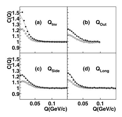
Figure 1.10:  $\pi^-\pi^-$  correlation function as measured by the STAR experiment at  $\sqrt{s_{NN}} = 130\,\mathrm{GeV}$  [52]. The open and solid points are before and after Coulomb correction, respectively.
