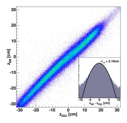
Figure 4.1: Correlation of the location of the primary vertex determined from BB and ZDC timing differences before event selection. The one-dimensional distribution is fitted with a Gaussian and its width is used for event selection. A  $3\sigma$  cut removes 1-3% of the events.
