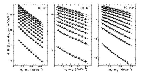
Figure 1.5:  $m_T$  spectra for  $\pi^{\pm}$ ,  $K^{\pm}$ , p and  $\bar{p}$  in  $\sqrt{s_{NN}} = 200 \,\text{GeV}$  Au+Au collisions at RHIC as measured by the STAR experiment [24]. The lower curve on each panel is p+p, while the other curves are Au+Au collisions at various centralities in the range 0-5% (top) to 70-80%. The pions are fitted with Bose-Einstein distribution  $\propto 1/(\exp(m_T/T)-1)$  while the kaons and protons are fitted with Blast-Wave distributions [22].
