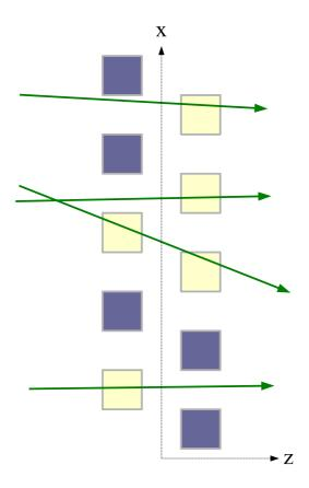
Figure 4.5: Several tracks intersecting a number of scintillator slats H1. The dark shaded slats have no hits.
